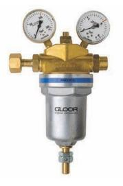
With working pressure and contents gauges and integral safety valve.With pipeaway facility fitted to safety valve for venting gases to<br/>atmosphere. Standard version with working pressure up to 10 bar. Also<br/>available with working pressure up to 20 or 30 bar (see below).Connection:screw connector (gas specific)Outlet:3/4", 1/2"Gases:A, AR, C, DL, H, HE, M, NH, NO, N,O, P and mixtures
